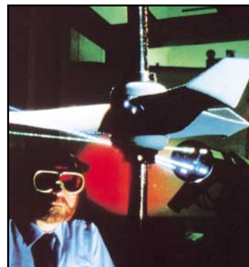
The LIGHTNIN laser can simultaneously measure flow, power, and mechanical load. A computer controls all the tests and displays the results.
