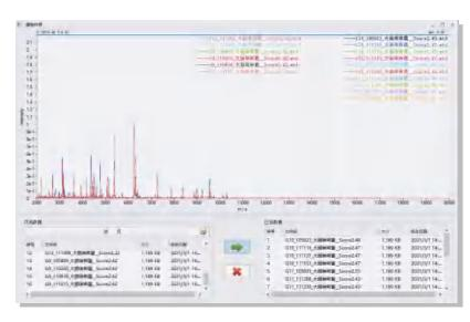
The system can intelligently identify and correct the  $\pm 10$  Da of the spectrum offset with synchro nous searching during the process. And the detection result will be obtained within 0.1s.
